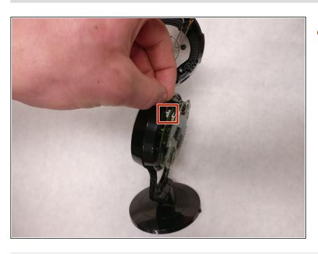
Detach the speaker wire by gently pulling on the side closest to the body of the camera.
