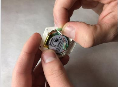
Remove the green tape shrouding the battery connector.
