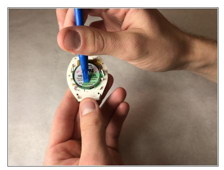
On the back cover use a plastic opening tool to remove the green tape retaining the battery.
