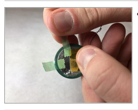
Remove the green tape on the back of the battery, it can be reused later.
