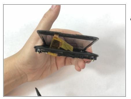
Pull screen away from frame making sure the ribbon cable stays attached.
