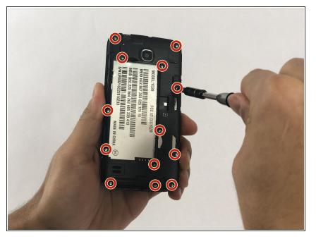
Remove the thirteen 3mm Phillips #00 screws from the back panel.
