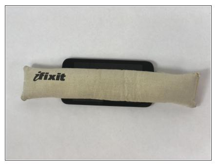
• Using an iOpener heat source tool, warm the screen of the phone to loosen adhesive of the screen.
