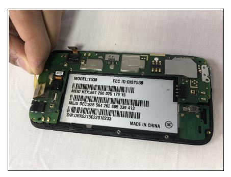
• Firmly hold the second ribbon cable's plastic film cover and pull up to disconnect.
