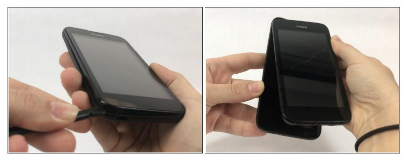
• Wedge your thumb nail, or the flat end of a spudger, into the bottom left corner and pry off.
