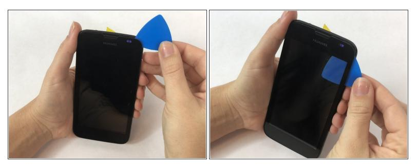
• Wedge an opening pick underneath the screen and slowly work your way around the screen.
