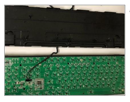
Pull apart the two parts of the panel to expose the motherboard and keys.
