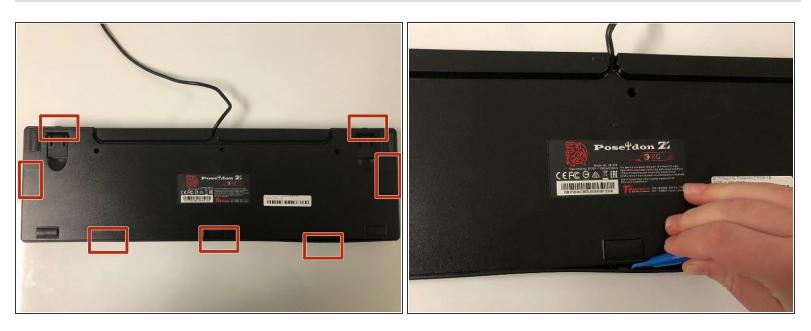
Pry at these points with a plastic opening tool to unclip the two halves of the keyboard case.
