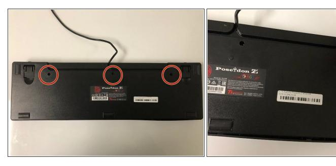
Remove the three JIS #1 screws from the back cover.
