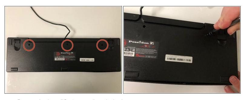
Remove the three JIS #1 screws from the back cover.
