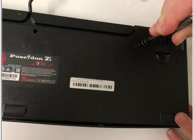
Remove the three JIS #1 screws from the back cover.
