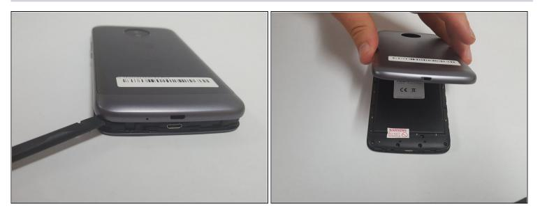
• Insert the spudger into the notch on the corner of the phone and lift up to remove the back case.
