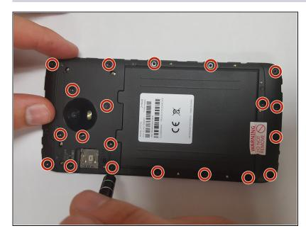
• Use the <u>T4 Torx Screwdriver</u> to remove the <u>17 3.2 mm screws</u> in the back panel covering the battery.
