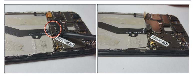
• Use the <u>Spudger</u> to lift up and detach the <u>Main Flex Cable</u> from the <u>Motherboard</u>.
