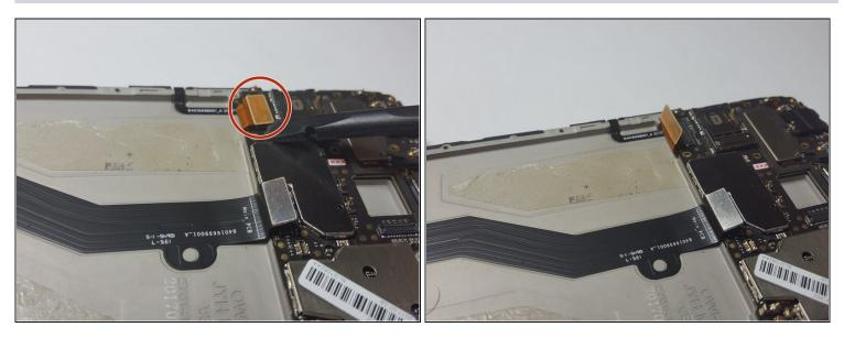
• Use the <u>Spudger</u> to lift up and detach the <u>LCD Screen Flex Cable</u> from the <u>Motherboard</u>.
