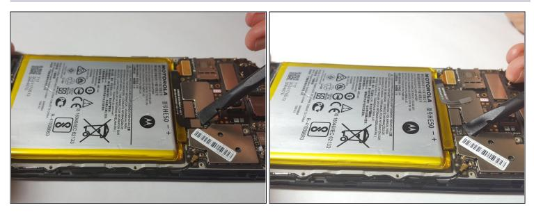
• After removing the back panel, use the spudger to lift and detach the <u>Battery Flux Cable</u> from the <u>Motherboard</u>.
