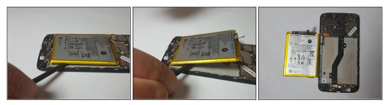
• Wedge the spudger between the battery and the phone to lift the battery up and remove the battery. There will be slight resistance to this but the battery will not be damaged by this. It is just the adhesive tape.
