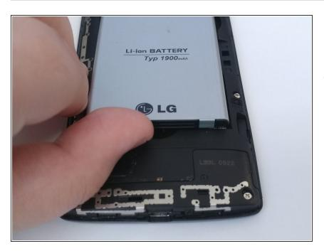
Place your thumb along the bottom of the battery and pry upwards to remove.
