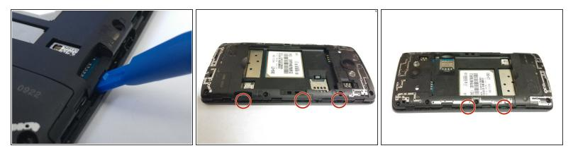
Use an opening tool on the marked locations to lift the edges up. There should be a small click when lifting these edges up.
