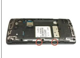
Use an opening tool on the marked locations to lift the edges up. There should be a small click when lifting these edges up.
