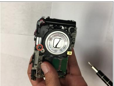
Remove the two 3mm Phillips #000 screws.
