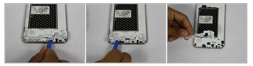
• Using a plastic opening tool, remove the antenna extender from the bottom.
