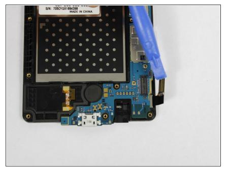
Disconnect the LCD from the motherboard with a plastic opening tool.
