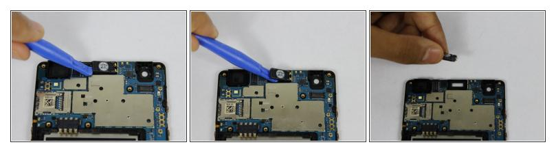
• Using a plastic opening tool, pry up the front facing speaker and remove it from the phone.
