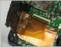
Lift the button board gently to reveal the ribbon connector.
