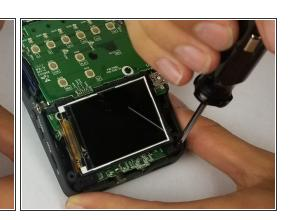
Unscrew three (PH #1), 7 mm screws (two on right side of display and one on the bottom left).
