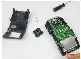
With the bottom of the device on a table, lift the top of the device and gently place it aside.
