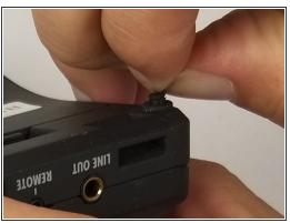
With device facedown, lift the four rubber feet from the device using tweezers or fingernails.
