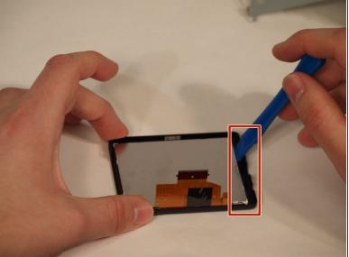
• The screen is glued into the casing. Remove the screen by carefulyl lifting along the edges of the case until the screen pops out. Place new screen into the existing casing. A small about of glue or adhesive may be necessary if their isn't sufficient adhesive remaining in the case. Repeat steps in reverse to reapply screen.
