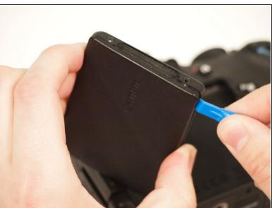
Following the removal of the 6 screws, Locate the joint of the casing. Place a flat lever inside this crevice and apply pressure. The case should simply pop open into the 2 casing pieces and the screen mechanism. Warning. No Dot try to remove bottom casing until next step.
