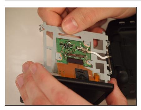
Now that the ribbon is disconnected, remove the board carefully and place it aside. This piece still works so leave it attached to camera.
