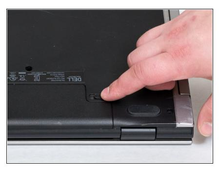
Slide both lock latches to the unlocked position.
