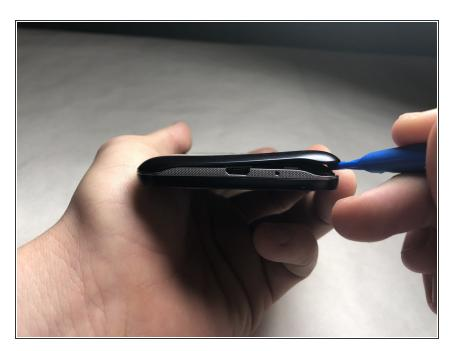
Wedge the plastic opening tool into the seam between the plastic backing and the rest of the phone.
