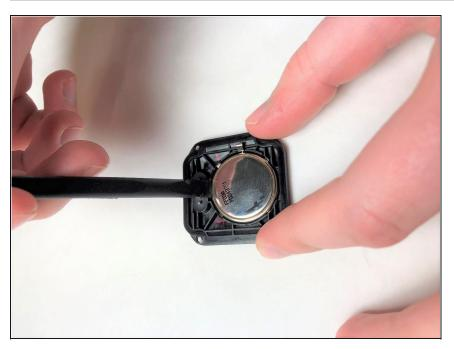
Pry the old battery out using a plastic spudger.
