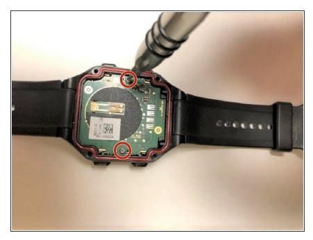
Unscrew the two T4 6 mm screws located on both sides of the motherboard.
