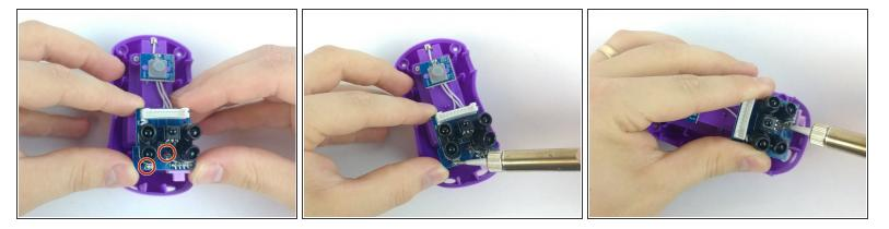
To remove the sensors, use a soldering iron to solder the two points and remove the red and black wires from the reverse side.
