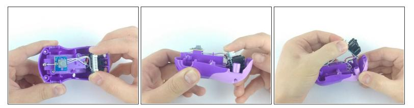
• For easier access to the sensor, tilt and pull the sensor away from the body.
