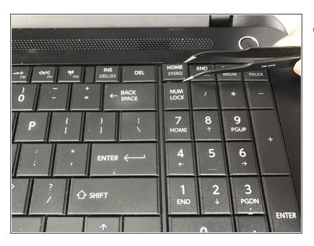
Align the key onto the keyboard
