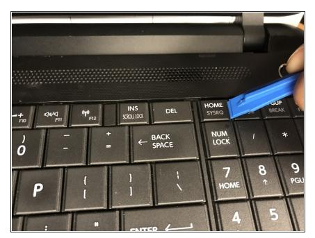
Use a plastic opening tool to lift a key off of the keyboard
