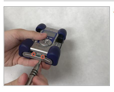
Using the Philips screwdriver, remove the bottom 2 screws (2.5mm).
