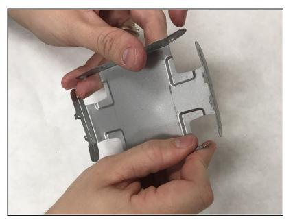
• Remove metal surround from the Jukebox. You may have to straighten out tabs that were bent during disassembly.
