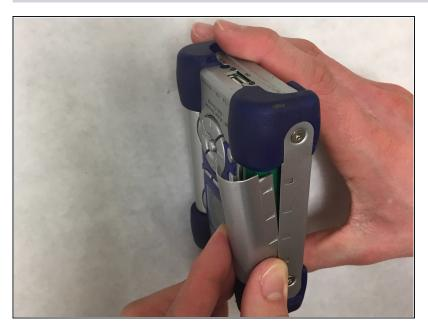
• Remove the plastic cover over the batteries on both sides of the device.
