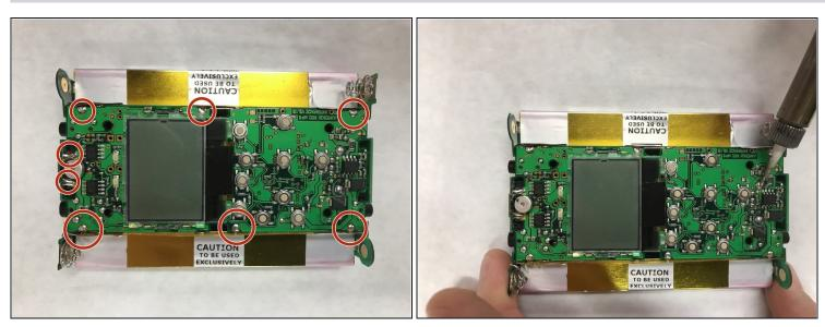
Desolder the motherboard from the frame at the eight locations shown. You may need to use a <u>desoldering pump</u>.
