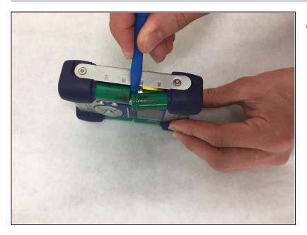
• Remove the batteries (may require a plastic opening tool or spudger to pop the batteries out).
