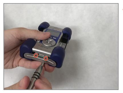
• Using the Philips screwdriver, remove the bottom 2 screws (2.5mm).
