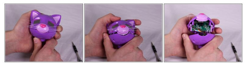
Hold the top and bottom halves of the head in each hand separately and gently pull away from each other to separate both halves.
