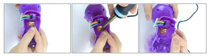
• Using a soldering Iron, carefully heat the solder point around the silver wire and pull gently until the wire lifts free.
