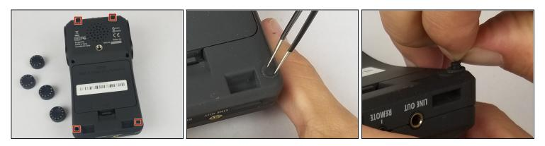
• With device facedown, lift the four rubber feet from the device using <u>tweezers</u> or fingernails.
