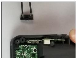
Use tweezers to lift the power switch out and set aside.
