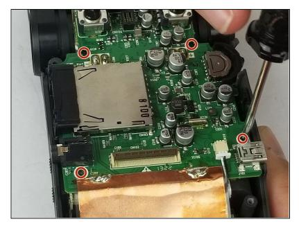
Unscrew four (PH #1), 8mm screws from the motherboard.
