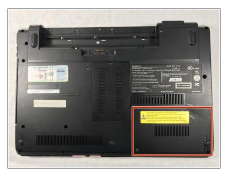
The hard drive panel is located in the bottom right corner of the device.
