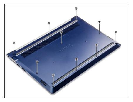
Remove the screws that secure the back cover to the computer
