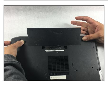
While still pushing in the tabs, using your pinky finger, lift the battery out of the laptop.
