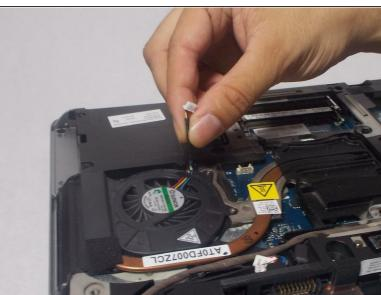
Use the plastic opening tool to unclip the connector.
