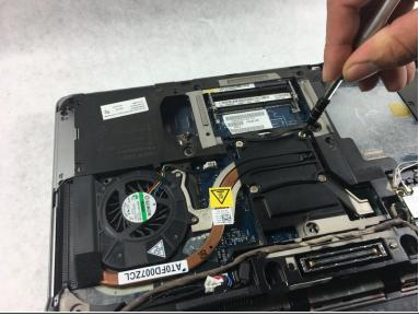
Using the screwdriver, remove four 10mm Phillips #0 spring screws from the fan assembly.
