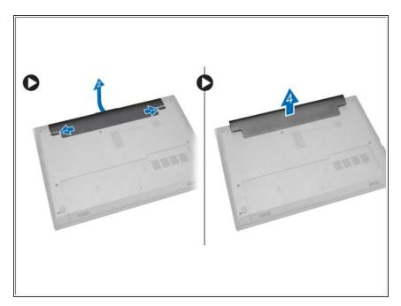
Slide the release latches outwards to unlock the battery and lift the battery to remove it from the computer.
