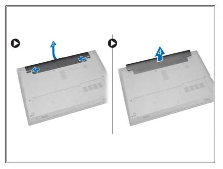
Slide the release latches outwards to unlock the battery and lift the battery to remove it from the computer.
