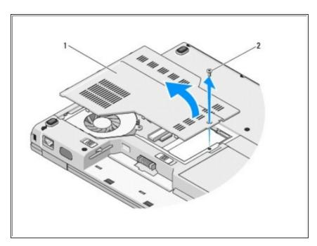
• Remove the M2.5 x 5-mm screw that secures the memory cover, and remove the cover and set it aside.
