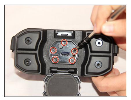
Then, proceed to unscrew the 5 Phillips #00 bit type, 9mm long screws located on the face of the charging dock.
