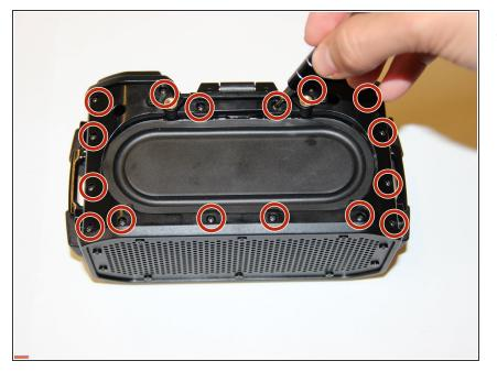
To remove the inner plastic casing, use a Phillips #00 head bit to remove the 16 small 9mm screws surrounding the top side of the device.
