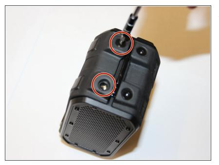
To remove the outer casing, use a 3mm Hex bit to remove the 4 large 12mm Hex screws on both sides of the device.
