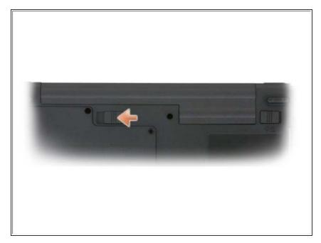
Slide the battery-bay latch on the bottom of the computer, and release.
