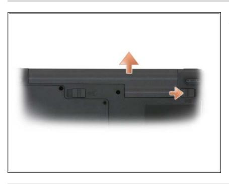
Slide the battery-bay latch release closest to the side of the computer, and then remove the battery from the bay
