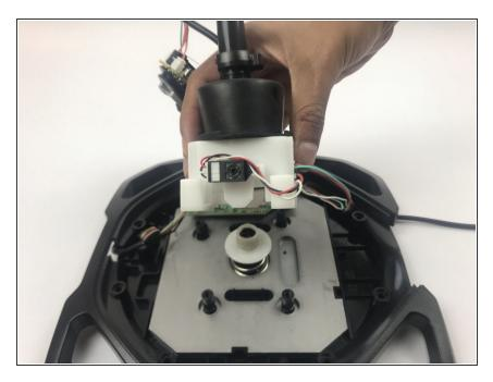
• Remove the joystick assembly.
