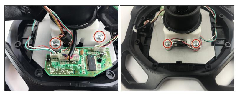
Remove the four 10mm Phillips #1 screws from the joystick base.
