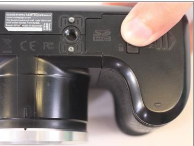
Slide switch to open lock position.
