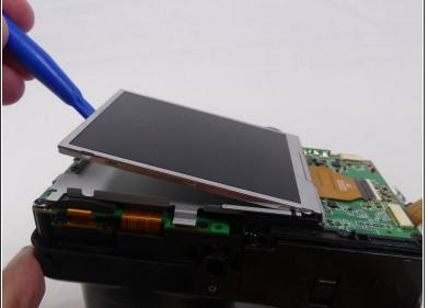
Pry the LCD screen out of the metal housing plate with a plastic opening tool.
