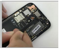
• Use the flat end of a spudger to disconnect the rear-facing camera connector from its socket on the mother board.
