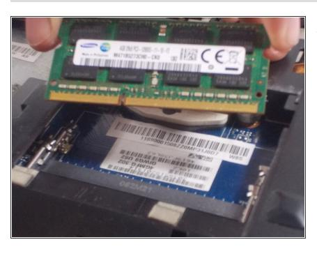
Carefully slide the RAM straight out of its socket. To reassemble your device, follow these instructions in reverse order.
