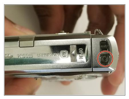
Remove the single Phillips #000 screw found next to the battery latch.
