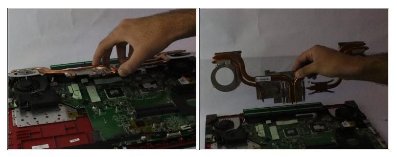
• Remove the cooling assembly by unscrewing the fourteen screws holding it in place.
