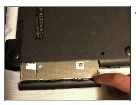
Gently slide the optical drive out of the side of the computer.
