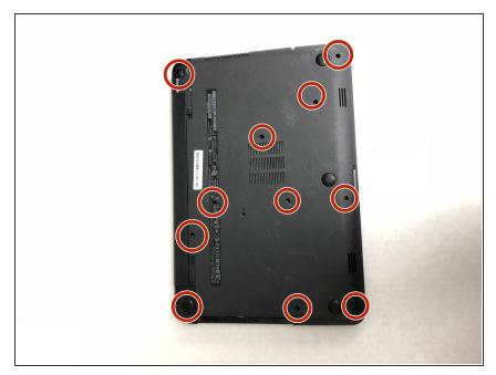
Remove the 11 small screws on the bottom of the computer that are shown in the picture.
