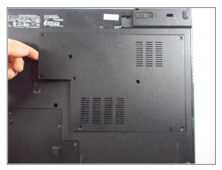
Lift back cover from the groove on the left side of the cover next to the symbol.
