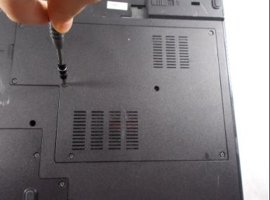
Unscrew the eight 6mm screws with a Philips #1 screw driver.
