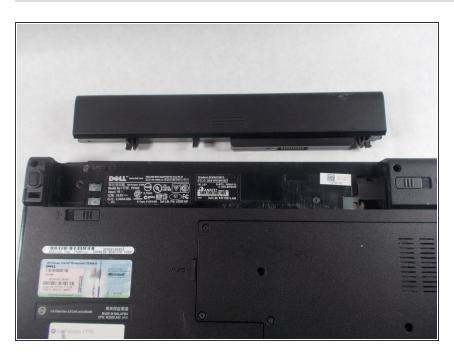
Remove the battery from the slot.
