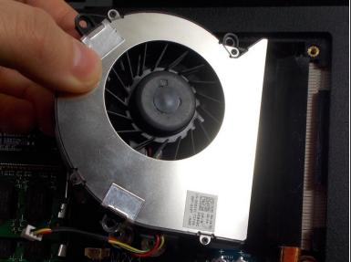
Gently lift and pull to the left until the fan is free from the heatsink.
