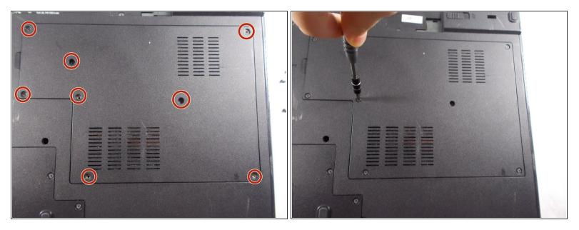
Unscrew the eight 6mm screws with a Philips #1 screw driver.
