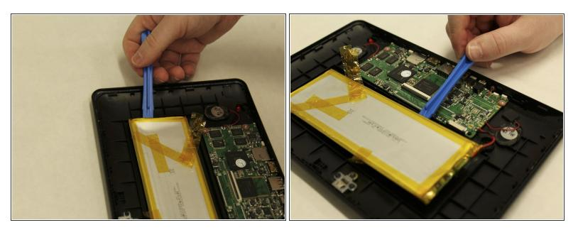
To remove the battery, use the plastic opening tool to pry one corner off of the battery and gently move the opening tool down to pull up one side of the battery.
