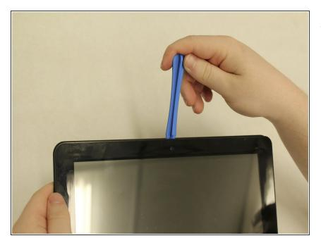
To begin, insert the plastic opening tool between the display and back cover and apply force until the back cover comes free from the device.
