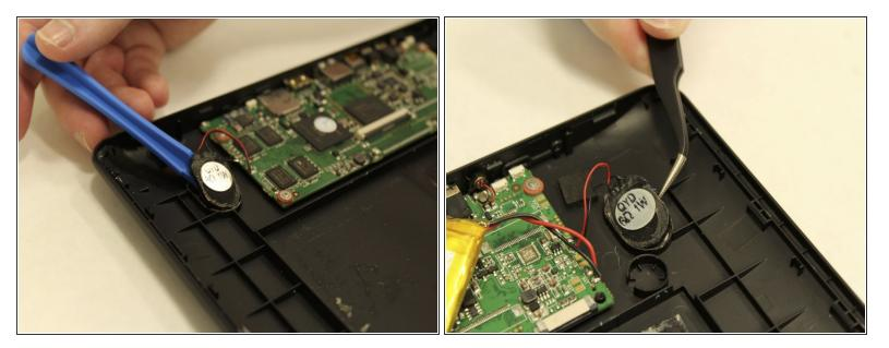
To remove the speakers, use the plastic opening tool to gently pry the speaker from the back cover, then use the tweezers to remove them fully.
