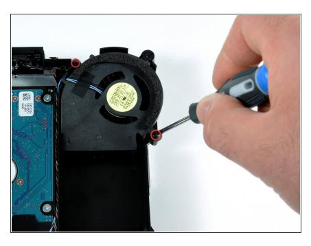
Remove the two Phillips screws securing the fan to the internal frame.
