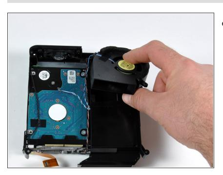
• Lift the fan out of the internal frame.
