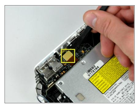
Use the flat end of a spudger to pry the audio ribbon cable connector up off the audio board.
