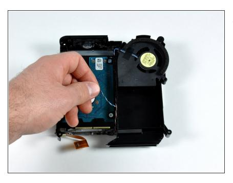
De-route the fan cable from the channel in the internal frame.
