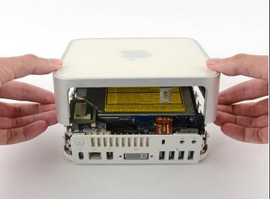
Flip the Mac mini back over and lift the top housing off of the lower housing.
