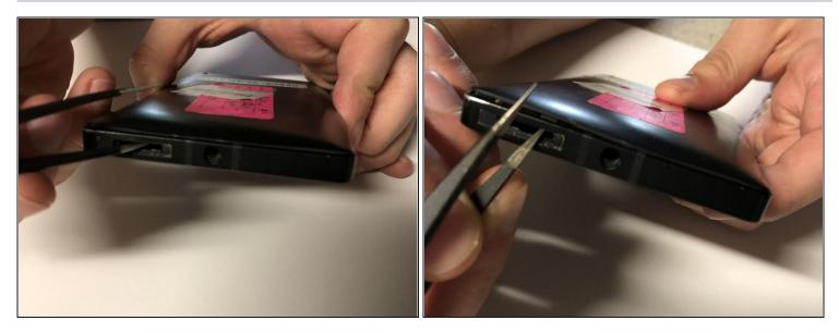
• Place <u>tweezers</u> or an opening tool in the SIM card slot and push upwards until the back panel pops out.
