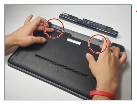
Slide the two release latches that were mentioned in the battery removal process to release the service panel.
