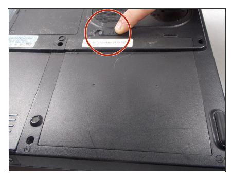
Locate the battery locking mechanism on the back side of the laptop. It is labeled with a lock and unlock symbol to indicate its function. The mechanism also has a serrated texture to increase grip.
