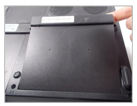
Pulling up with your right hand while the locking mechanism in in the unlocked position will release the battery from its socket.
