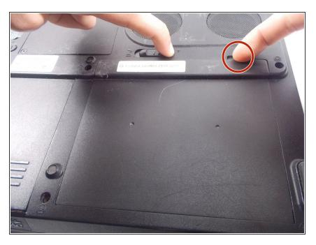
Place your left hand on the locking mechanism and slide it all the way to the left. This will move it into the unlocked position. While holding the mechanism in the unlocked position place another finger in the cavity to the right of the locking mechanism.
