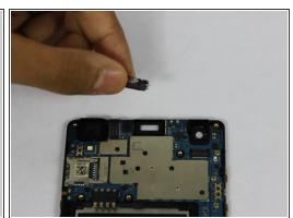
Using a plastic opening tool, pry up the front facing speaker and remove from the phone.
