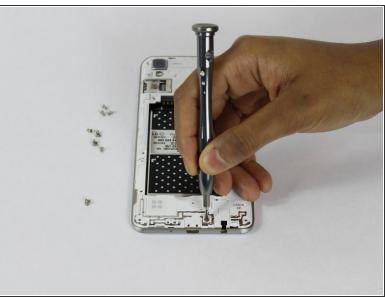
Remove the twelve 2mm JIS #00 screws from the mid-frame.
