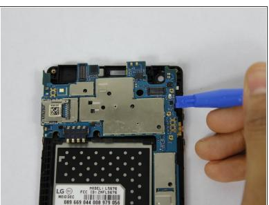
Use a plastic opening tool to pry up the motherboard and pull out to remove.
