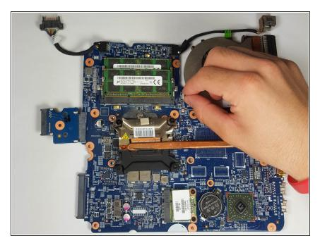
Disconnect the small cable that connects the fan to the motherboard.
