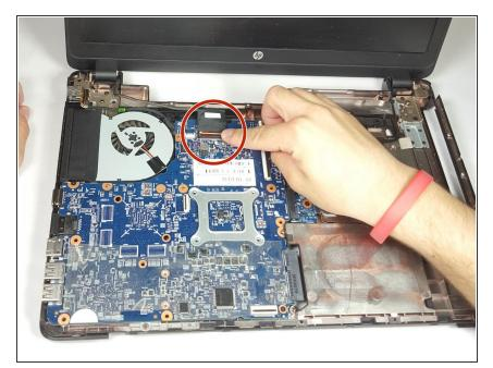
Disconnect the ribbon attached to the motherboard
