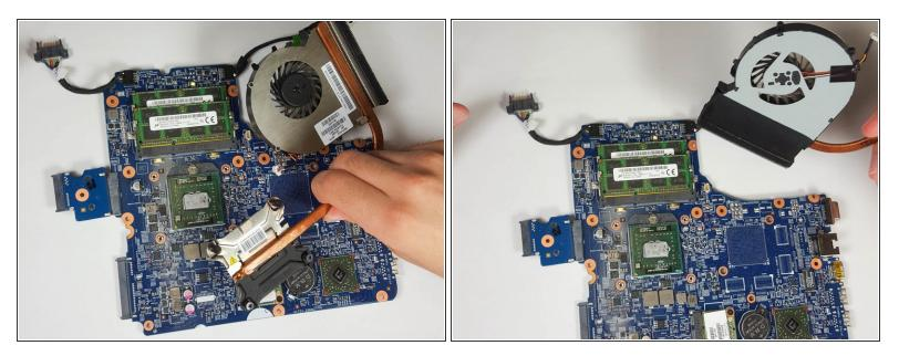
• Lift the fan from the motherboard to fully remove it.
