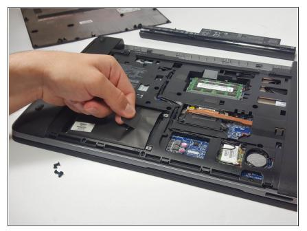
• Pull the hard drive cover tab to the left in order to disconnect the hard drive from the computer.
