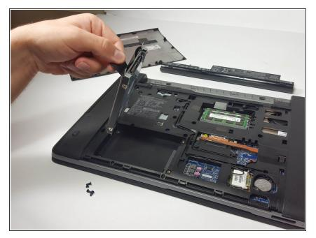
• Finally, using the same tab, lift the hard drive out of the hard drive port.
