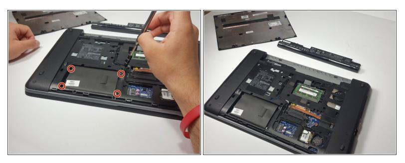
Using a Phillips #0 Screwdriver, remove the four Phillips 3 mm screws that secure the hard drive into the computer.
