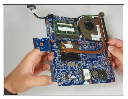
• Turn the motherboard over and lay it flat so that the copper "L" is visible.
