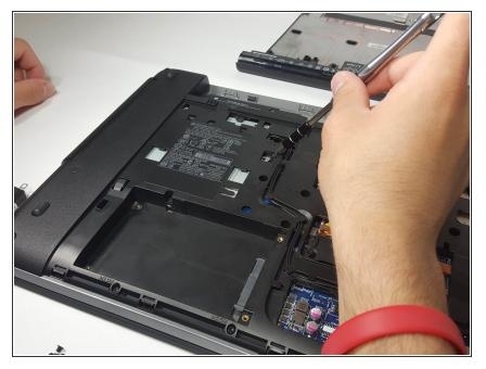
Using the screwdriver, gently push the silver tab that the screw secured to the left to release the DVD/CD drive from the computer.
