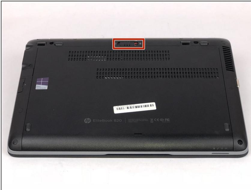
**!** Ensure the laptop is completely powered off and power adapter is unplugged before removing the battery.
