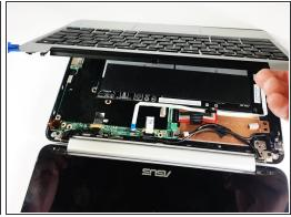
Pry the palm rest assembly apart from the bottom cover using a spudger. This step may require
