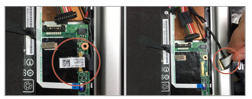
Disconnect the LCD cable from the motherboard using the pointed end of a plastic spudger.
