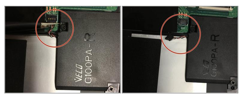
• Disconnect the speaker cable from the motherboard using the pointed end of a plastic spudger.
