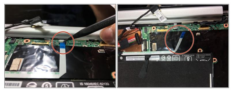
Disconnect the motherboard to powerboard cable from the motherboard using the pointed end of a plastic spudger.
