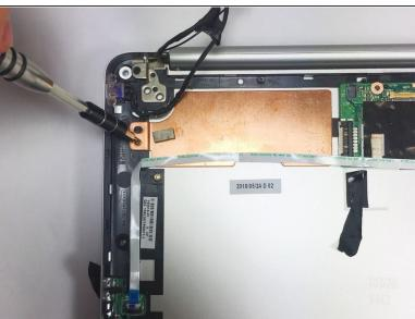
Remove the five 2.7mm motherboard screws with a T5 screwdriver.
