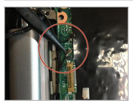
Disconnect the two WiFi antenna cables from the motherboard using the pointed end of a plastic spudger or simply by pulling the cables apart from the motherboard with your fingers.
