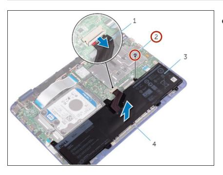
Replace the screw that secures the battery to the palm-rest and keyboard assembly.
