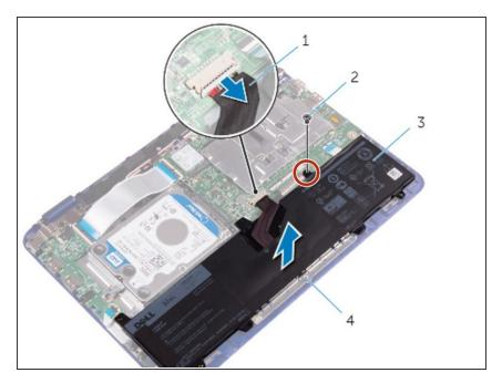
Align the screw hole on the NEW battery with the screw hole on the palm-rest and keyboard assembly.
